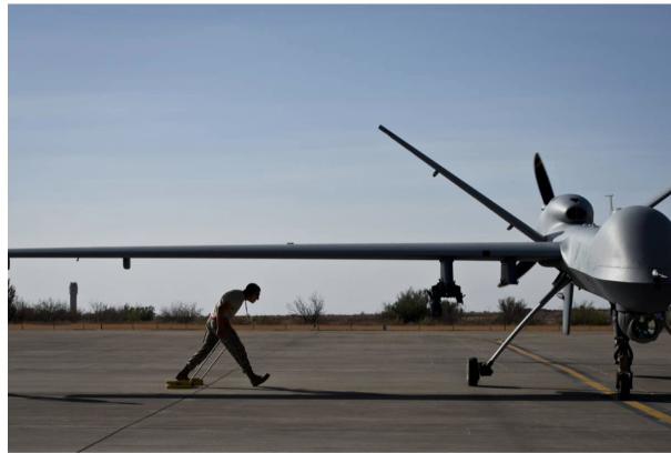
After taxiing in an MQ-9 Reaper, Airman 1st Class Jon Mann walks under a Reaper's wing to place wheel chocks to prevent accidental movement April 24, 2013 at Holloman Air Force Base, N.M.
